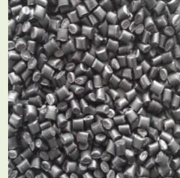
Zylindergranulat : PA6 / PA6.6 / PP-GF / PP-TV / PP-EPDM / ABS
